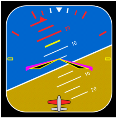
Fig. 8 Roll angles greater than the EPS maximum are red, and the roll indicator is red because the maximum roll angle is exceeded.
