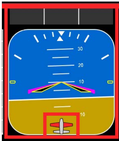
Fig. 20 Ice accretion notification with severe wing ice (red) shown. The ambient strip (red) flashes and surrounds the aircraft icon to capture the attention of the pilot.
