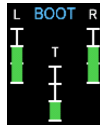
Fig. 13 De-ice boots status display. Wing de-ice boots are on medium, and tail de-ice boot is on low.
