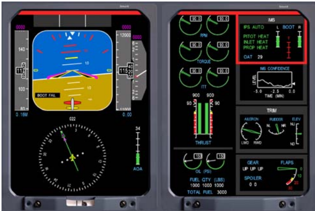
Fig. 6 Ambient strip (red) showing boot failure.
