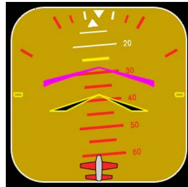
Fig. 12 Pitch up command given by the flight director (purple) since the minimum pitch angle is reached.
