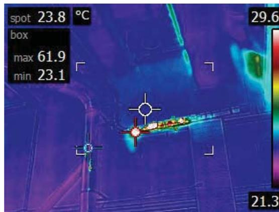
Figure 6. A thermal infrared image of the rolling rig motor after 30 seconds of full power.
