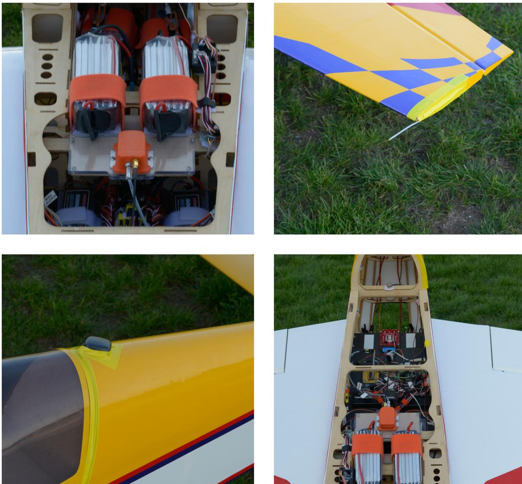
**Figure 12.** The avionics suite components, starting on the top left and going clockwise: a) the IMU is mounted as close as possible to the CG, b) the pitot probe is mounted on the left wingtip, c) the GPS antenna is mounted atop the fuselage behind the canopy, and d) the rear balsa/carbon fiber sandwich tray with the flight computer, autopilot, IMU signal conversion board, and two regulators.
