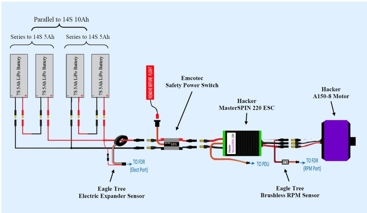
Figure 8. A propulsion system diagram for the Aero Testbed unmanned aircraft.
