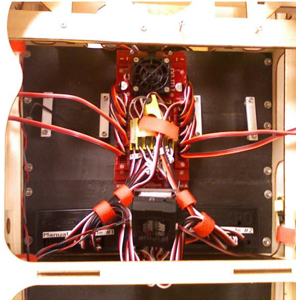
**Figure 7.** Smart-Fly power distribution unit, JR receiver, and 2irc manual overrides installed on the front balsa/carbon-fiber sandwich tray.
