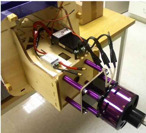
Figure 9. The Hacker A150-8 brushless motor (bottom right), MasterSPIN 220 electronics speed controller (top middle), and SPS safety switch (center left) seen before the cowling, propeller, and spinner were installed.
