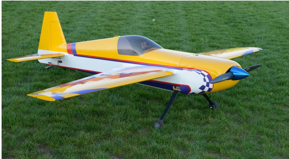
**Figure 1.** A photograph of the UIUC Aero Testbed, which is an electric unmanned 35% scale Extra 260 aerobatic aircraft with a 105 in wingspan, a weight of 37 lb, and is instrumented with an avionics suite that includes a 6-DOF inertial measurement unit, GPS receiver, and pitot probe among other sensors.
