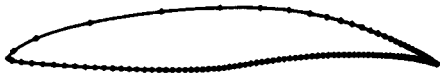
Fig. 12 Cascade blade of Fig. 10 with symbols plotted at each of the 120 points to illustrate point spacing.
