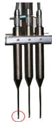
Figure 12. Three Cobra Probes. Probe head is circled in red.
