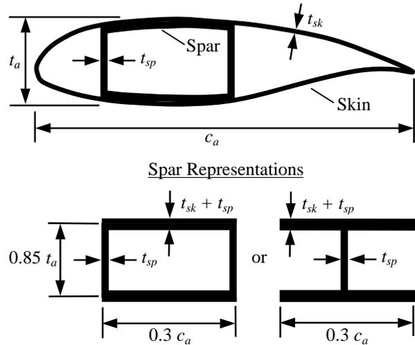
Fig. 1: Modeling of the airfoil section.
