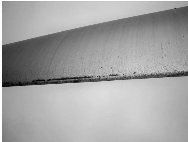
Figure 12. Leading edge of a wind turbine blade exposed to erosion (courtesy of 3M).
