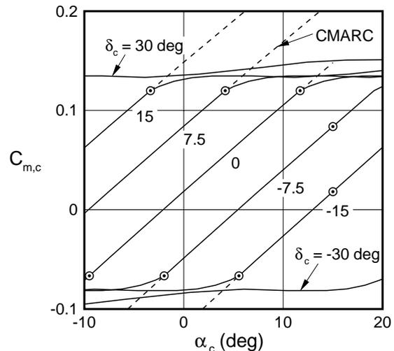
Fig. 14 Pitching moment coefficient versus angle of attack for the 1903 canard at canard deflection angles ranging from  $-30$  to  $30$  deg.
