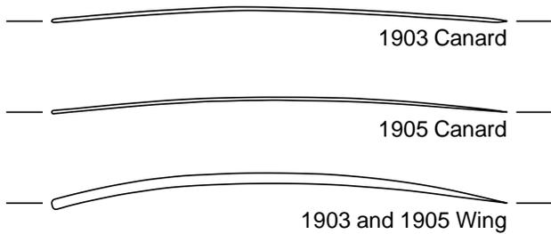
Fig. 5 Airfoils used for CMARC panel mesh.
