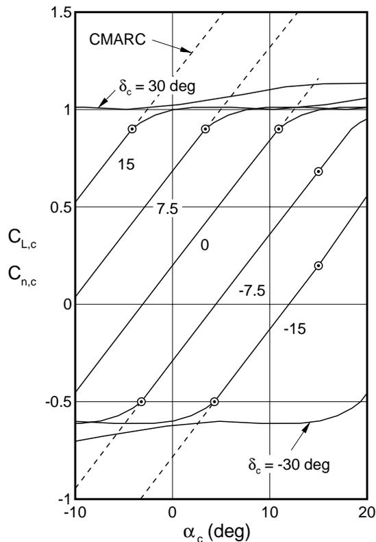
Fig. 18 Lift coefficient versus angle of attack for the 1905 canard at canard deflection angles ranging from  $-30$  to  $30$  deg.
