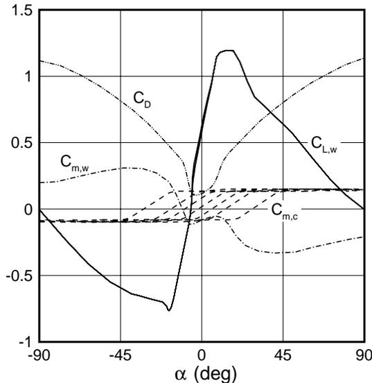
Fig. 16 Aerodynamic coefficients for the 1903 Flyer from  $-90$  to  $90$  deg angle of attack.
