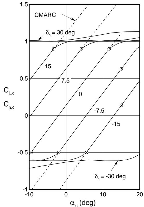
Fig. 13 Lift coefficient versus angle of attack for the 1903 canard at canard deflection angles ranging from  $-30$  to  $30$  deg.
