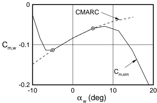
Fig. 12 Pitching moment coefficient versus angle of attack for the main biplane wing of the 1903 Flyer.
