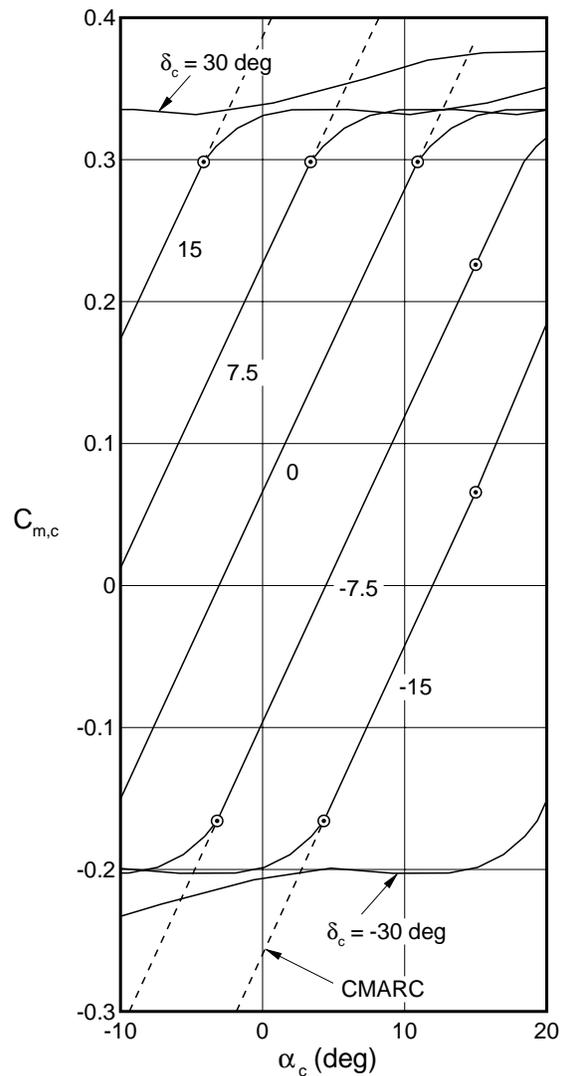
Fig. 19 Pitching moment coefficient versus angle of attack for the 1905 canard at canard deflection angles ranging from  $-30$  to  $30$  deg.
