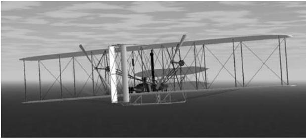
Fig. 15 View of the 1903 Wright Flyer with a 30 deg canard deflection in FlightGear.
