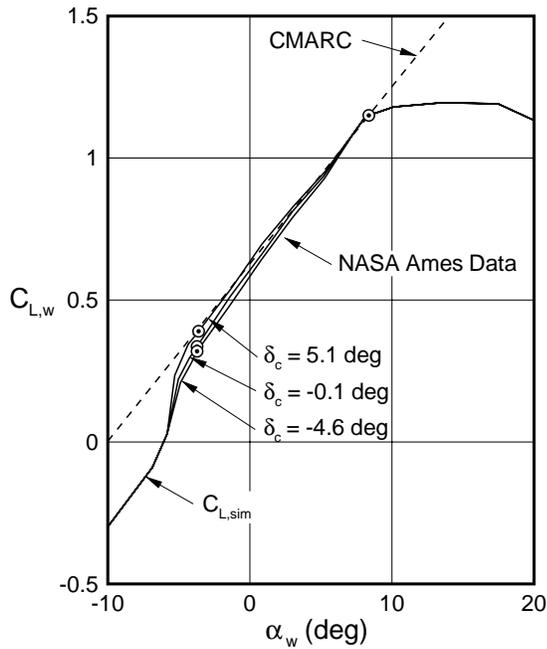
Fig. 11 Lift coefficient versus angle of attack from CMARC and wind tunnel tests for the main biplane wing.
