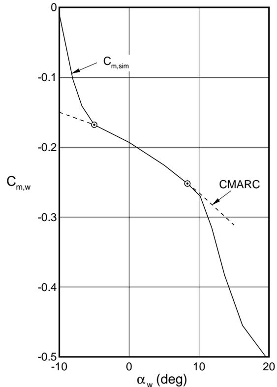
Fig. 17 Pitching moment coefficient versus angle of attack for the main biplane wing of the 1905 Flyer.
