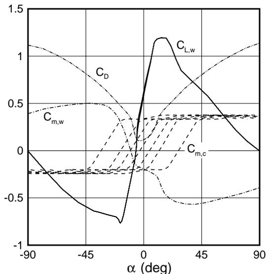
**Fig. 20 Aerodynamic coefficients for the 1905 Flyer from  $-90$  to  $90$  deg angle of attack.**
