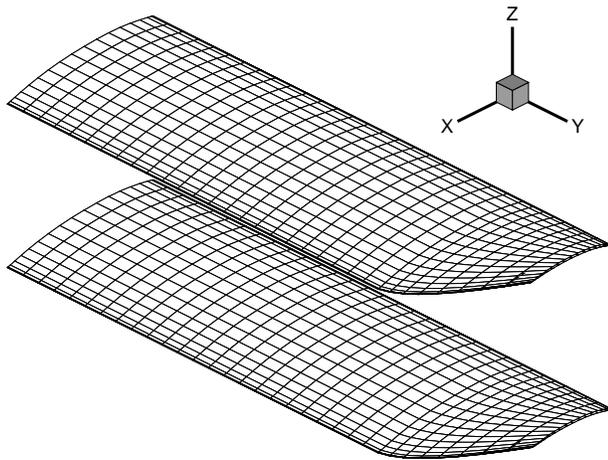
Fig. 6 Mesh for the 1905 wing.
