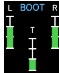
Fig. 13 De-ice boots status display. Wing de-ice boots are on medium, and tail de-ice boot is on low.
