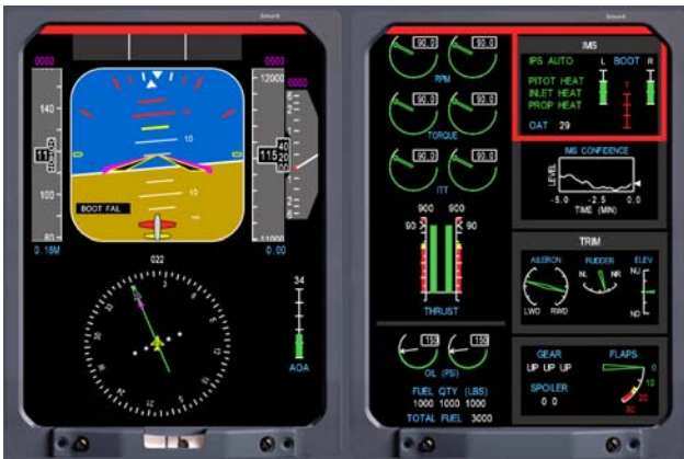
Fig. 6 Ambient strip (red) showing boot failure.
