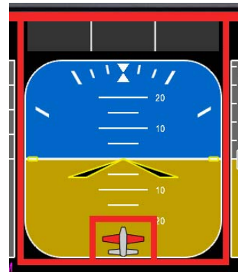
Fig. 4 Ice accretion notification (wing ice shown). The red ambient strip flashes and surrounds the problem area (in this case a small airplane icon showing ice), while an auditory alert provides additional pilot cues.
